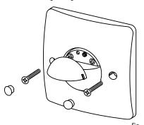
Additionally to the horizontal detection plane the Indoor 180 has a vertical detection plane which detects also movements underneath the motion detector. In order to prevent detection within the vertical range of coverage, apply the cover.
