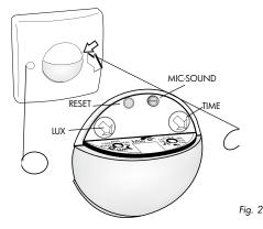
Lux-level, microphone and timer can be set here: remove top cover as shown, this will give access to the controls. Please follow the markings on the flat top of the lens for adjustment.
